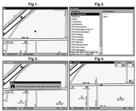
Sequence for setting a waypoint. Fig. 1: While traveling, press WPT twice to call up the Find Waypoint screen (Fig. 2) and set a point. Fig. 3: A message says the waypoint has been saved. Fig. 4: vehicle continues on its way; the waypoint number is visible on map.
